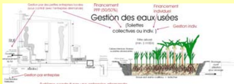
Urine diverting concrete slab Greywater garden
