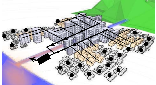
Conventional Wastewater System
